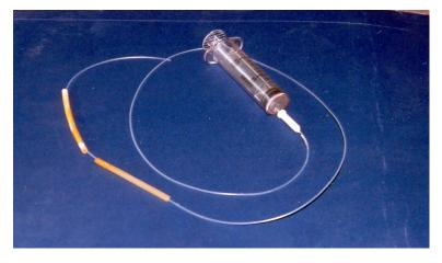
To empty the cane you can either tap the bottom on the bench and shake the mercury down or, more successfully use the ubiquitous catheter . These are plastic tubes which come in 2 or more diameters to enable entry into different bore sizes of cane. They have a collar which fits a standard plastic syringe. Obtain one or more pieces of hard plastic tube (the orange ones in this picture) which are threaded onto the catheter and into the short arm of the cane. These larger tubes
