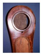
The hygrometer housing at the top was very badly damaged and the bezel and glass missing. I purchased a nice quality ready-made bezel from Barometer World but it was too small in diameter to fill the hole. Therefore I decided to use imagination and after patching in the hygrometer keyhole I made a ring housing as shown on the left. The bezel fits into the hygrometer with a
