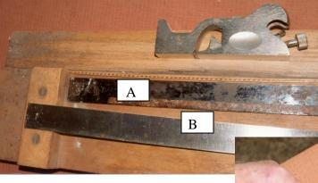
The one-sided stringing was then glued into the vacant areas, taped down, warmed with a hot air gun and tapped firmly into shape :
