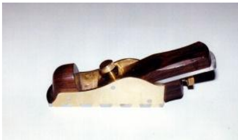
Image 12. New quality adjustable block plane by Karl Holtey with steel sole dovetailed to gunmetal sides and very nice rosewood infill and thick parallel blade. Just simply the best modern plane money can buy.
