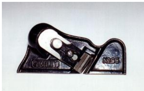
Image 11. A more unusual Stanley (USA) 95 edge trimming plane. Initially used for truing up man-made boards before veneering.
