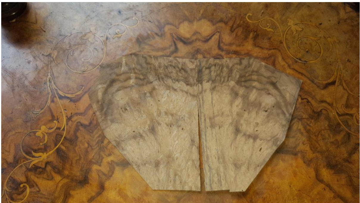
The veneers were then carefully placed to line up as best possible with the original walnut figuring
