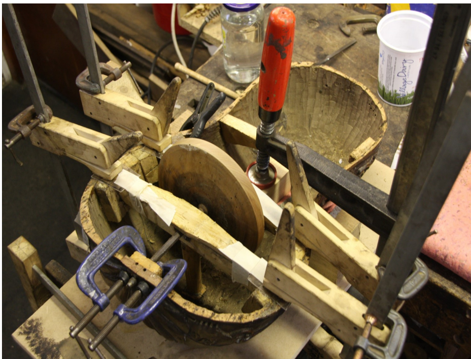
Once the individual parts of the mechanism had been restored they were all re-assembled and re-fitted to the body of the instrument. Alignment had to be absolutely precise; the cross members set such that the wheel would always run perpendicularly to the strings. Rather than using the usual scotch animal glue, much slower setting fish glue was utilised in order to allow time for fine adjustment before clamping up.
