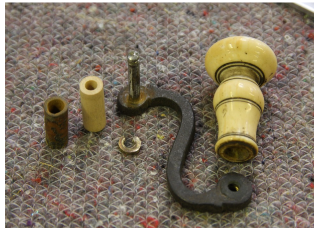
The beautiful ivory handle had become sloppy upon the crank mechanism; this was wholly dismantled, the handle bushed and riveted upon its arbour.
