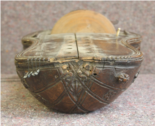
Here we can see the split down the centre of the table due to shrinkage caused by the timber drying out
