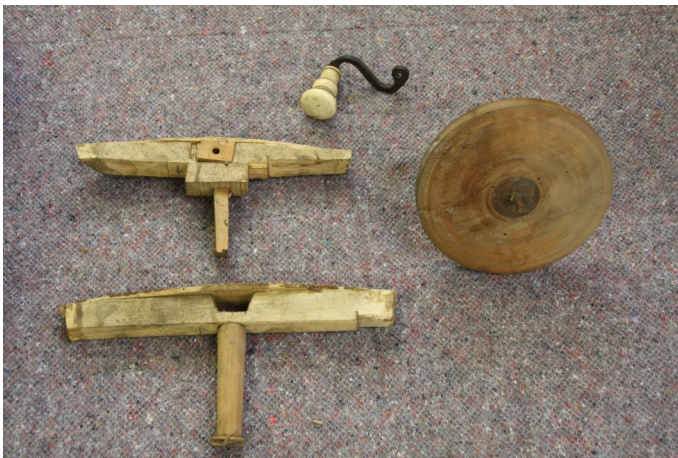
The cross members, once removed, were consolidated and any wear to the pivots taken up to facilitate the true running of the wheel.
