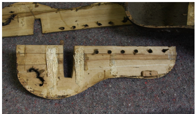
The table came off in two parts. Significant further worm damage can be seen to the cross struts, part of which has come adrift whilst still attached to the underside of the table.
